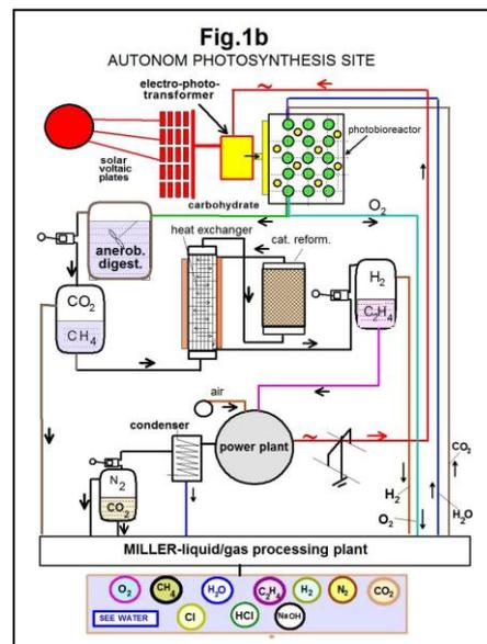
This captive carbon reaction cycle is closed by recycling the carbon dioxide produced in the photosynthesis and bio-digestion steps and the generated electric current in the combustion step for the purpose of irradiation in the photosynthesising stage.
