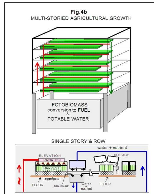
**Fig.4b** illustrates schematically a space saving and highly automated system for the same photosynthesising purposes.
